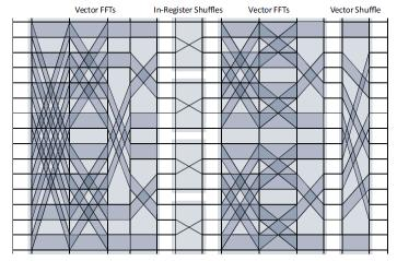
$\Big(\big((\mathrm{DFT}_2\otimes I_2)T_2^4(I_2\otimes \mathrm{DFT}_2)L_2^4\big)\otimes I_2\Big)\otimes I_2\Big)T_4^{16}\Big(I_2\otimes (L_2^4\otimes I_2)(I_2\otimes L_2^4)\big((\mathrm{DFT}_2\otimes I_2)T_2^4(I_2\otimes \mathrm{DFT}_2)L_2^4\big)\otimes I_2\Big)\Big(L_2^8\otimes I_2\Big)$
