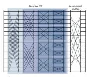
$\left(\mathrm{DFT}_2\otimes I_8\right)T_8^{16}\left(I_2\otimes\left((\mathrm{DFT}_2\otimes I_4)T_4^8\left(I_2\otimes\left((\mathrm{DFT}_2\otimes I_2)T_2^4(I_2\otimes\mathrm{DFT}_2)L_2^4\right)\right)L_2^8\right)\right)L_2^{16}$
