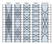
$\left( \left( I_1 \otimes \mathrm{DFT}_2 \otimes I_8 \right) D_0^{16} \right) \left( \left( I_2 \otimes \mathrm{DFT}_2 \otimes I_4 \right) D_1^{16} \right) \left( \left( I_4 \otimes \mathrm{DFT}_2 \otimes I_2 \right) D_2^{16} \right) \left( \left( I_8 \otimes \mathrm{DFT}_2 \otimes I_1 \right) D_3^{16} \right) R_2^{16}$
