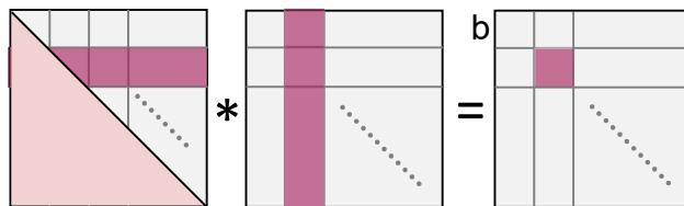
Figure 2: MMM with triangular matrix after blocking.
